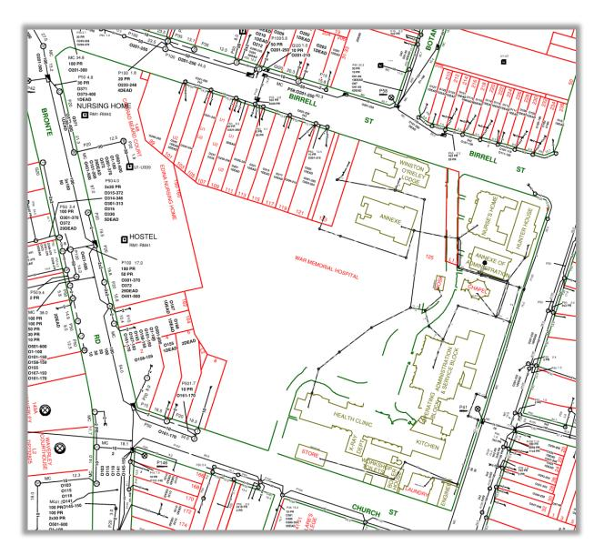
It is noted that Telstra's pit and conduit network extends into the eastern side of the site to supply the Hospital, Chapel, Nurses Home etc. Under the redevelopment it is would be preferred to retain this system to minimize disturbance and rework to the existing development.
