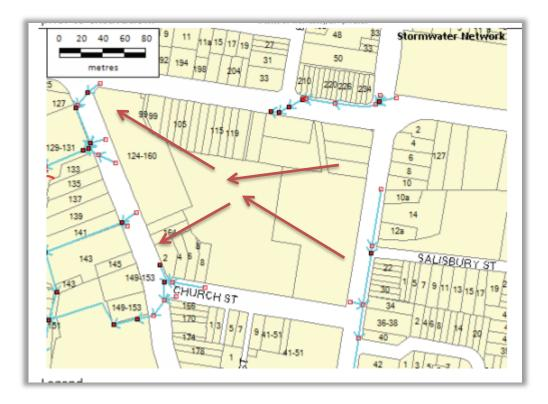
Also noted in the image above is the general arrangement arrows (red) of major stormwater infrastructure within the site. Due to the nature of the network within the site and the limited visual site inspection, a detailed survey would be required to confirm this information and any miscellaneous trunk main (s) not defined by the visual site inspection.
